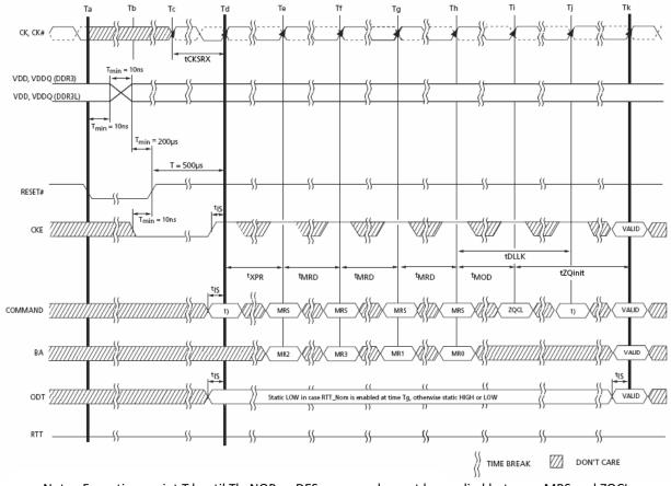
Note : From time point Td until Tk, NOP or DES commands must be applied between MRS and ZQCL commands
