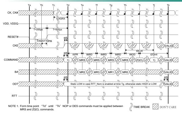
Reset and Initialization Sequence at Power-on Ramping
